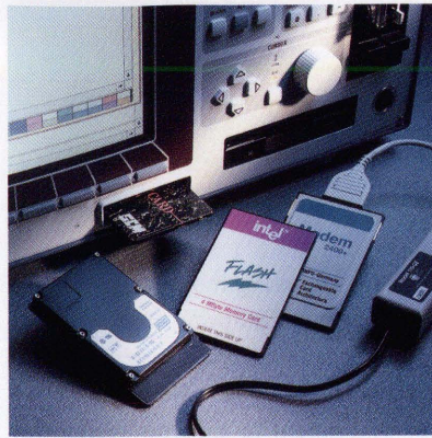
FIG 3 PSM storage media; front left: PCMCIA exchangeable hard disk Photo 41 498/1
