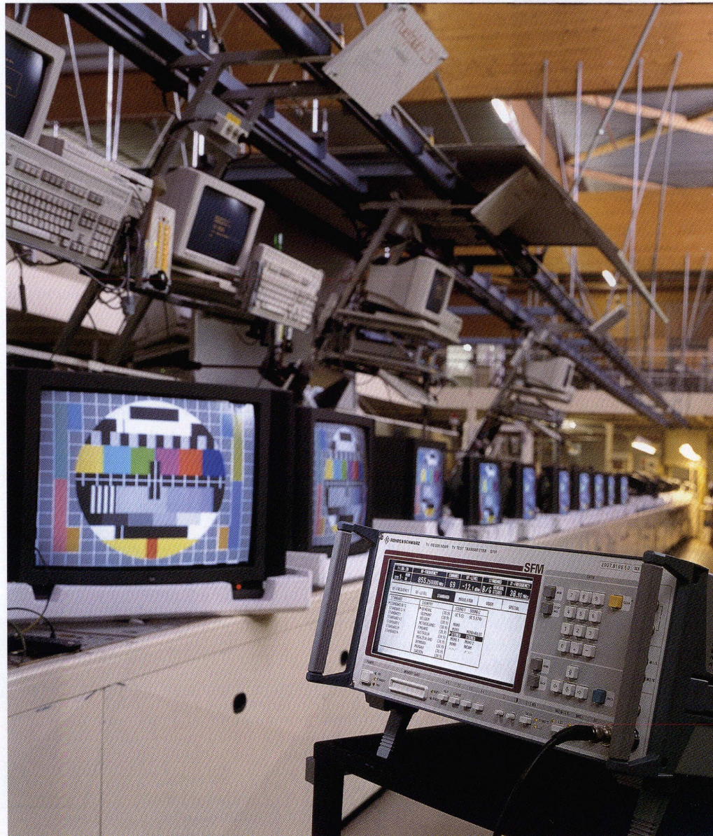
FIG 1 TV Test Transmitter SFM in TV-set production Photo 41 763/2
