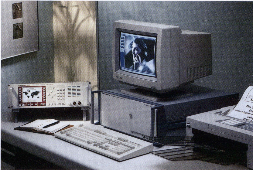
FIG 1 MERLIN system processor, data terminal for top-quality radioteletype networks (here with HF Transceiver XK 2100) Photo 41 268/2
